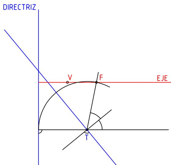
11.-DETERMINAR EL FOCO, EL EJE Y EL VERTICE DE UNA PARABOLA CONOCIDOS:
