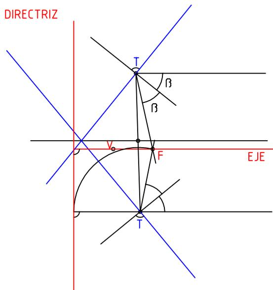
12.-DETERMINAR EL FOCO, EL EJE Y EL VERTICE DE UNA PARABOLA CONOCIDOS:
